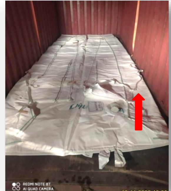
The belt tying must be 'taut but not tight'
