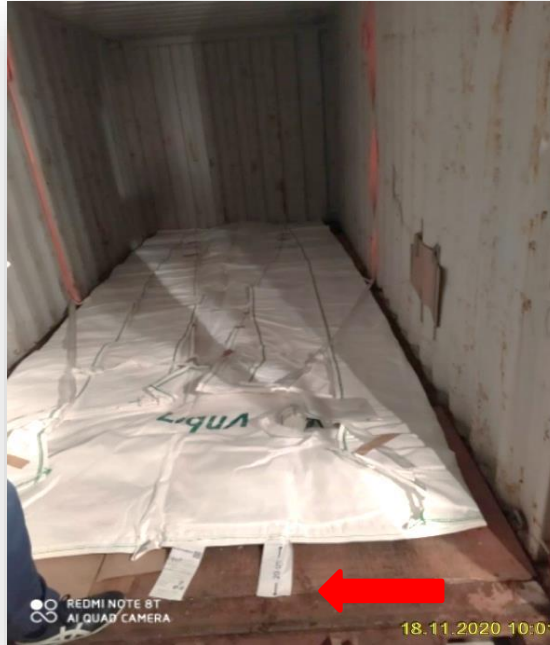
The distance must be 20 cm between the flexitank and the outer end of the container
