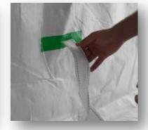
Use the big gap shown with blue circle to tie the belt to the lashing lug/ring. The ring is behind the Steam Liner. Use the gap to pull the belt and then tie to the ring.
