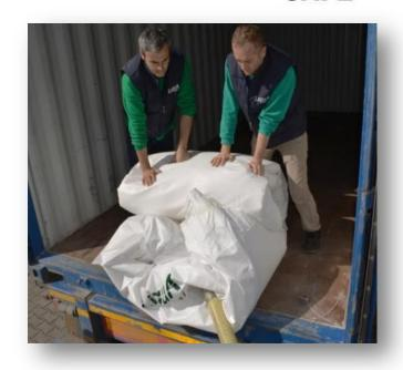
Until the Steam Liner lashing straps. Drain the condensed steam at the bottom of the Steam Liner before removing the flexitank.
