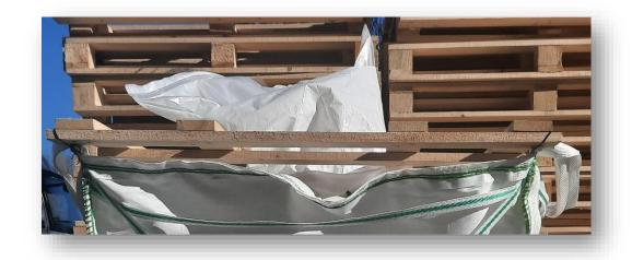
Pull out the filling flange of the inner liner as much as possible.
