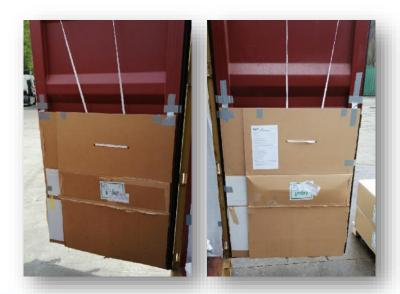
Bolts on the doors may damage the surface of K-Flex. Cover the sharp edges of the bolts with silicon and cover the doors with thick carton boards.
