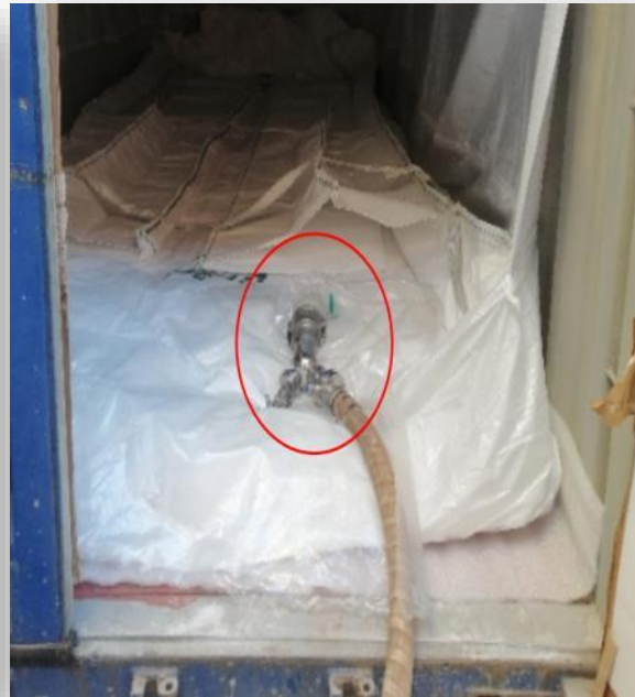
Use the flexitank bonnet to avoid possible contamination
