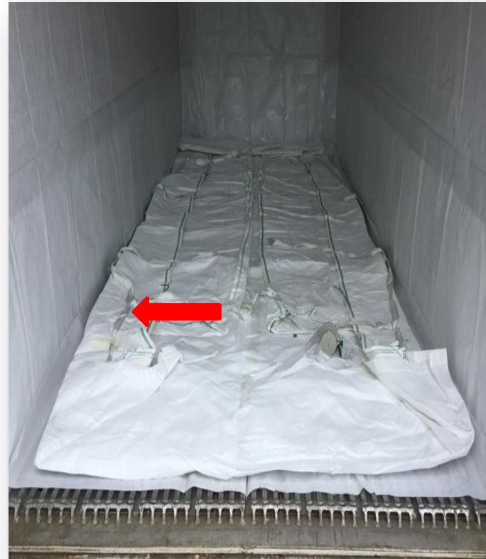
The belt tying must be 'taut but not tight'
